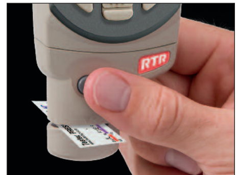
Align probe arrows with tape positioning dots
